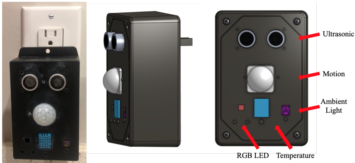
Figure: Sensor Station connected to Outlet (Left), CAD Model of Sensor Station (Middle and Right)
