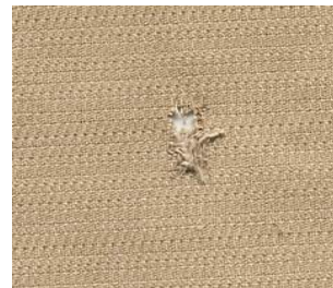
Fig. 6 Original Faulty (Hole) Fabric
