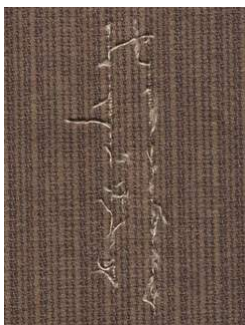
Fig. 4 Original Faulty (Scratch) Fabric
