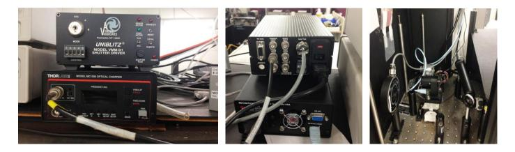
Thorlabs Model MC 1000 Optical Chopper EXT REF IN to Boxcar Trigger Light blue cable goes to physical chopper on table
