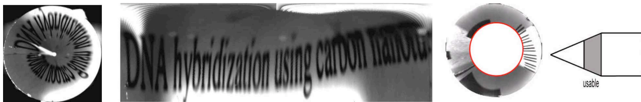
Fig. 6. Image distortion due to the conic mirror and software image reconstruction. Left: unprocessed image acquired through the side-looking optical imaging system; center: corresponding unwrapped image; right: illustration of the original unprocessed image and corresponding reflective surface on the conic mirror. The spatial resolution is degraded at the tip of the conical mirror (center portion of the original image on the left, top portion of the reconstructed image in the middle).
