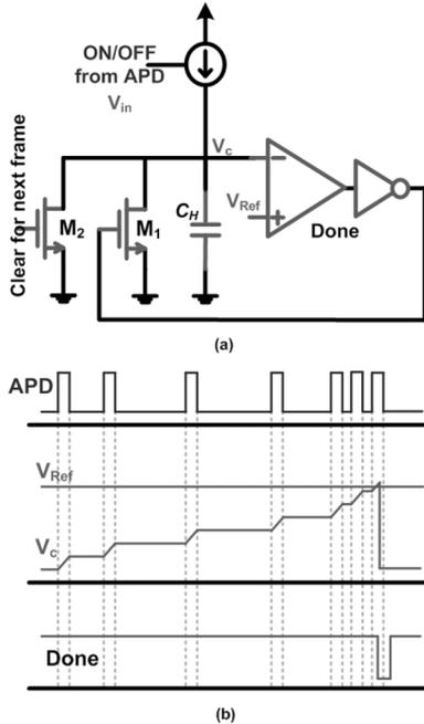
Fig. 3. (a) Schematic diagram of the designed analog counter. (b) Waveform of the operation of the analog counter.
