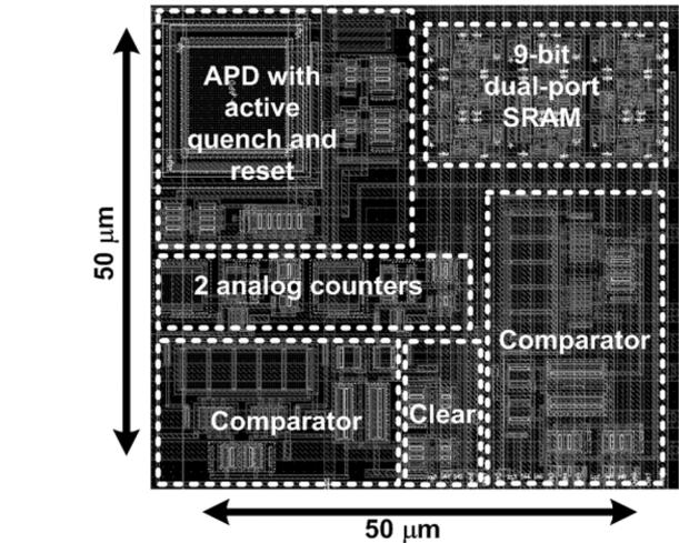
Fig. 5. Layout of a SPAD pixel with in-pixel analog counting and SRAM for parallel pixel analog-to-digital conversion.
