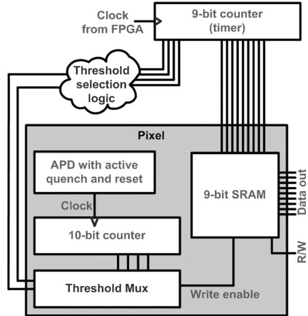
Fig. 2. Block diagram of the TDSPC pixel.
