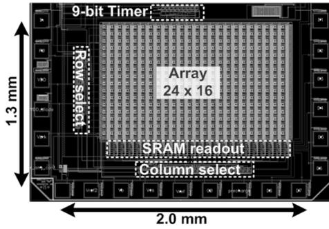
Fig. 6. Layout of the  $24 \times 16$  pixel TDSPIC with timer, readout, and array access circuits.
