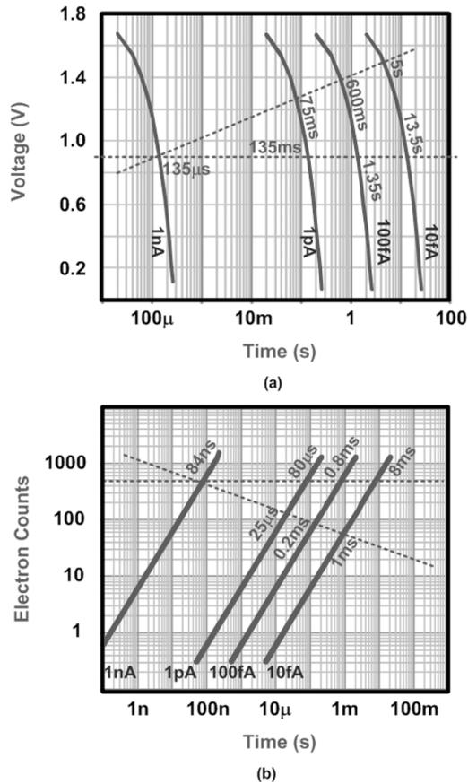
Fig. 1. (a) Calculated APS output voltage for four different optical signals showing the generated photocurrents and the corresponding times required to drop below the threshold voltage. (b) Electron count equivalent of (a).
