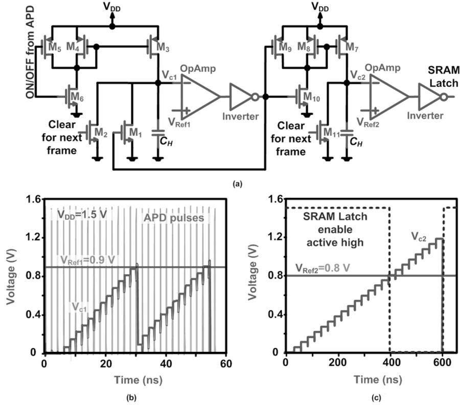
Fig. 4. (a) Two-stage analog counter schematic diagram and the simulation results of (b) the first stage and (c) the second stage showing the SRAM latch enable signal.
