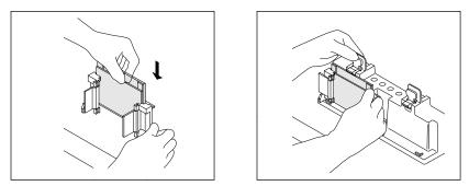
Fig. 2. Assembling the Mini-PROTEAN Tetra cell casting frame and casting stand.
