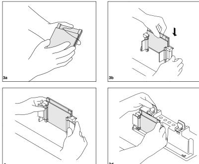
Fig. 3. Assembling the Mini-PROTEAN casting stand and frame.
