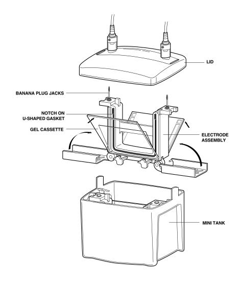
Fig. 1. Assembling the Mini-PROTEAN Tetra cell.
